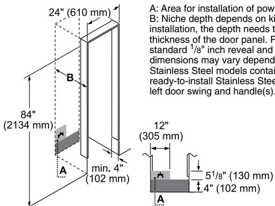
A: Area for installation of power connection.
