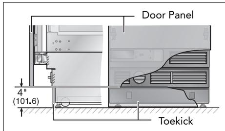
Typical 4" (102 mm) toekick height. Velcro adhesive strips are used to fasten the toekick to the appliance. Venting grille and (if applicable) the water filter cavity are located above the toekick area.
