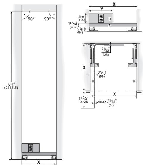
A: Area for running the water line. It is recommended the water-box be placed adjacent to the installation cutout, so that it can be accessed for service without uninstalling the appliance. If this is not possible, place the recessed water box adjacent to the power supply socket elevated at the heights as referenced in areas A+B.
