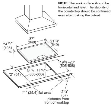
\* Minimum distance from cutout to the wall \*\* Recessed depth (includes 1" air clearance)
