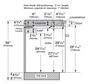
Note: Dimensions based on standard countertop height (36" with 43/4" toekick including base plate).
