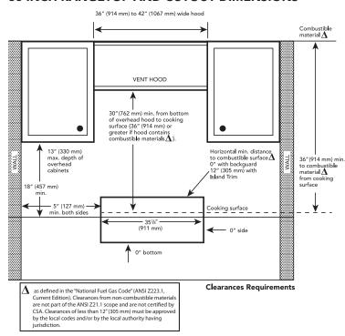
**NOTE:** A 36-inch minimum clearance is required between the top of the cooking surface and the bottom of an unprotected cabinet. A 30-inch clearance can be used when the bottom of the wood or metal cabinet is protected by not less than 1/4 inch of a flame retardant material covered with not less than No. 28 MSG sheet steel, 0.015 inch (0.4 mm) thick stainless steel, 0.024 inch (0.6 mm) aluminum, or 0.020 inch (0.5 mm) thick copper.
